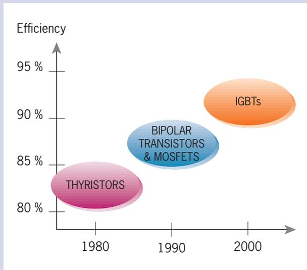
**A 15% increase in efficiency has reduced losses by a factor of 4 !**
